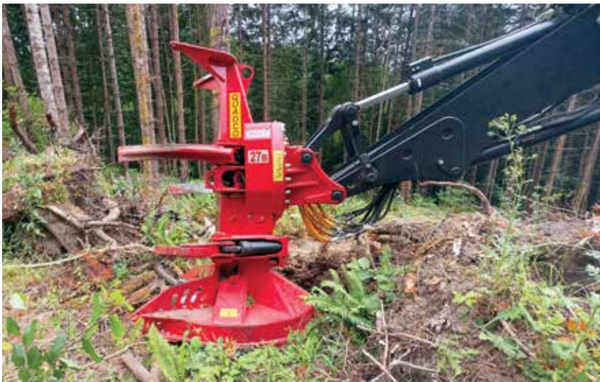
To cut up to 27-inch trees, TNB Mechanical Felling owner David White uses a Quadco 27B high-speed saw.
