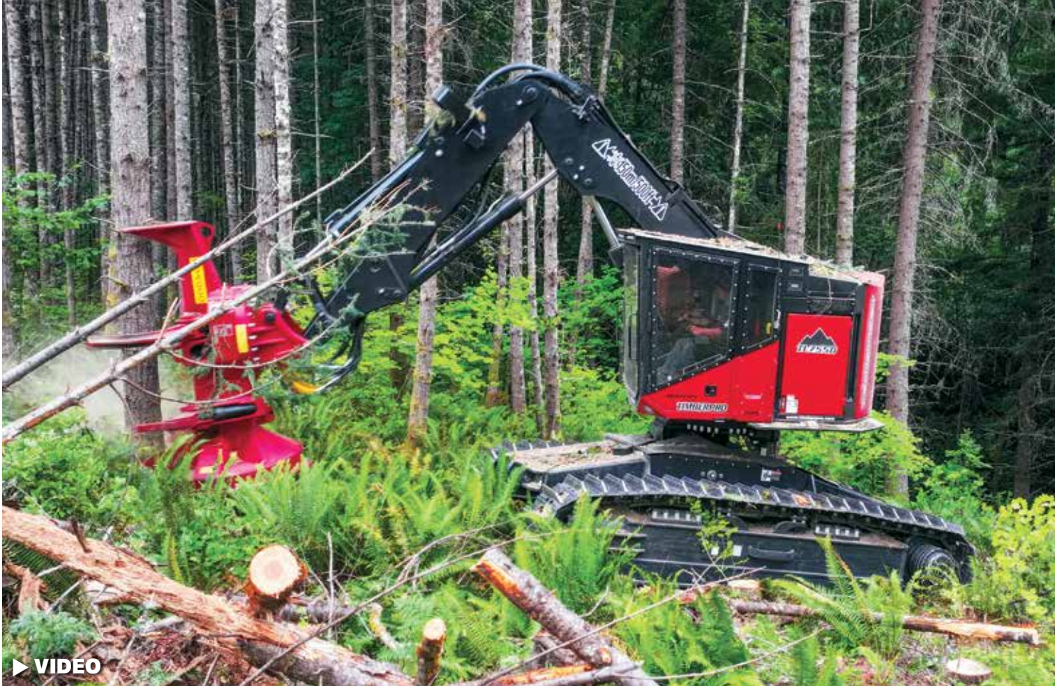
With a TimberPro TL755D West Coast Edition feller buncher, TNB Mechanical Felling owner David White cuts trees.
