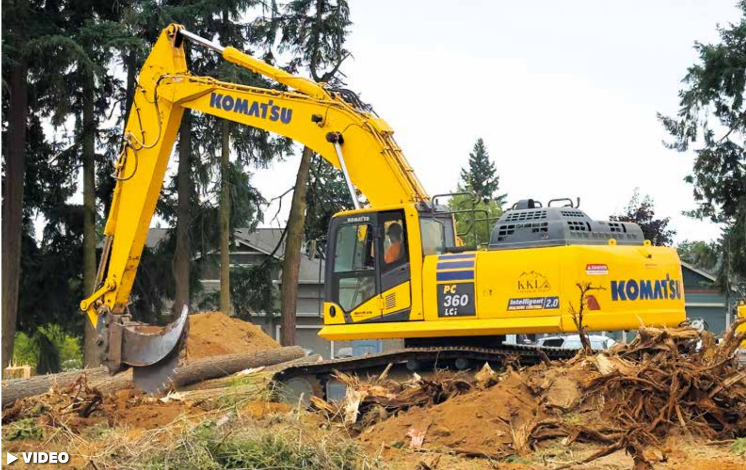
KKLA Contractors uses its Komatsu PC360LCi-11 intelligent machine control (IMC) excavator for a variety of tasks, including utility installation, tree and stump removal, mass excavation, and more.
