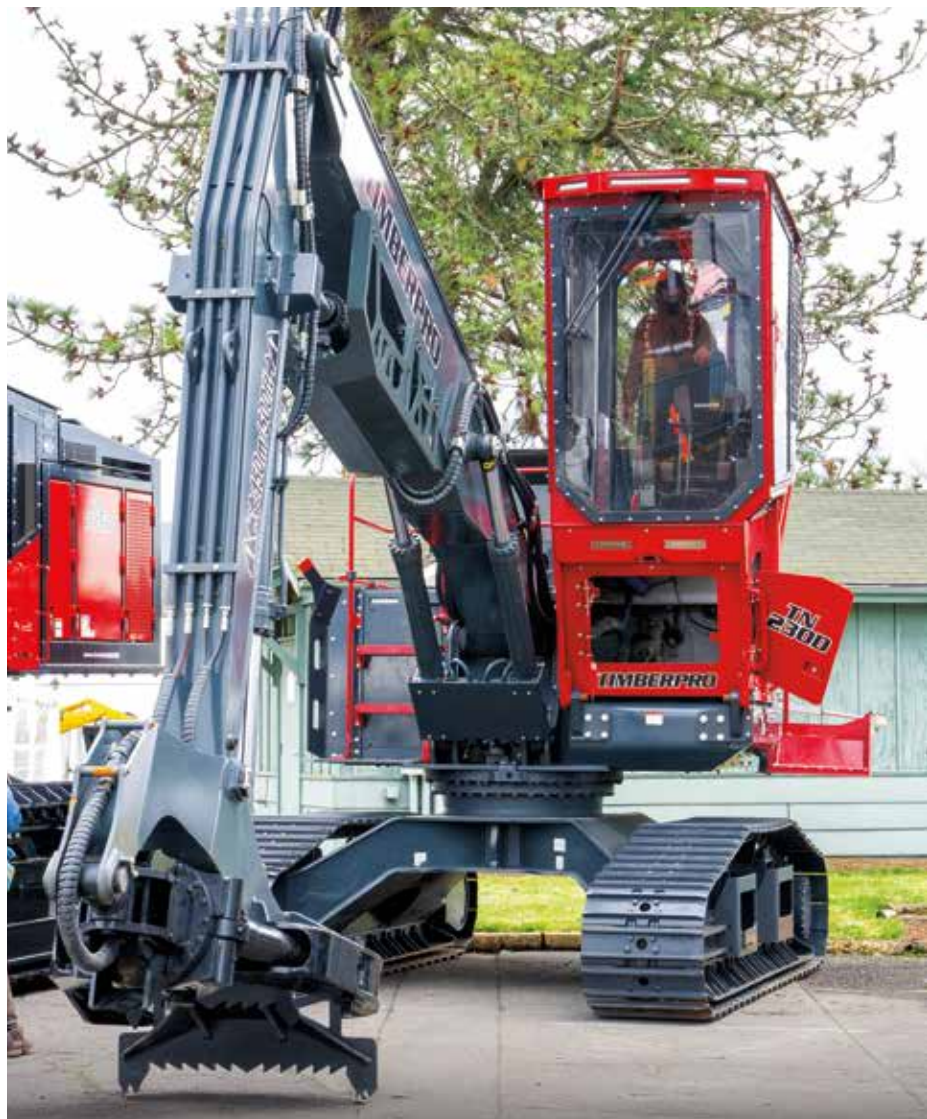
The TimberPro TN230D log loader offers a 36-foot reach and 58,244 foot-pounds of swing torque. It also features Power Max, which temporarily increases engine horsepower and hydraulic flow to support tough forestry tasks.
