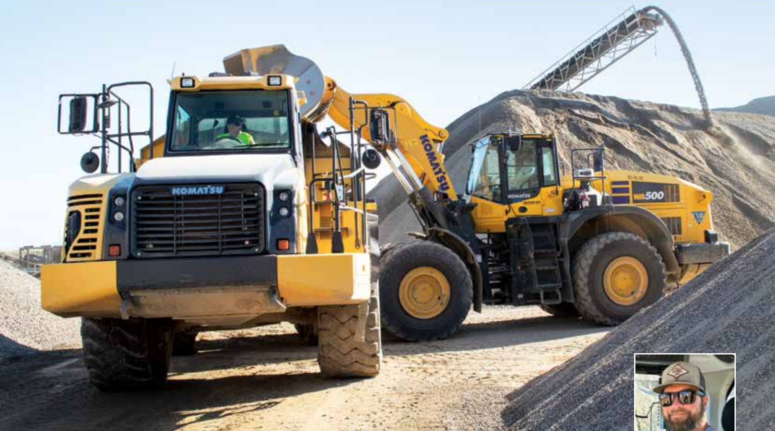
Operator Justin George loads a Komatsu HM400 articulated truck with a Komatsu WA500 wheel loader equipped with a 9-yard bucket and oversized tires. "The visibility is incredible," said George. "I love the extra-large bucket. It makes loading trucks a lot easier."
