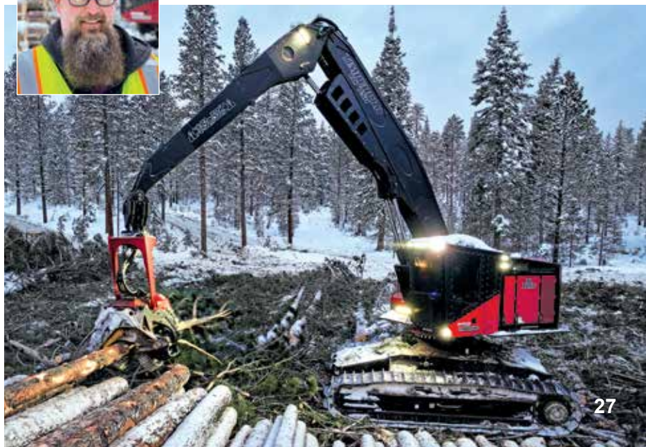
Operator Toby Winegar processes logs with a TimberPro TL775D tracked feller buncher on a job site near John Day, Ore. “It’s the most powerful machine I have run,” commented Winegar. “It allows you to do your job more efficiently.”
