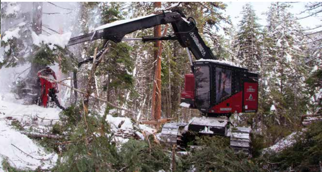
Operator Bob McConnell cuts and processes timber on a hillside with a TimberPro TL735D tracked feller buncher. "The self-leveling cab keeps you from having to strain to see what you are cutting or processing," noted McConnell.
